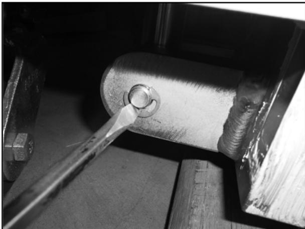
3. Remove E-clips from the pin at the bottom of the internal cylinder, and then remove the pin.
