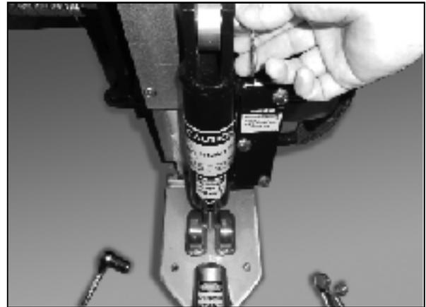
2. Remove the front cylinder by taking the 1/2" bolt out of the bottom and removing the pin from the top of the cylinder.
