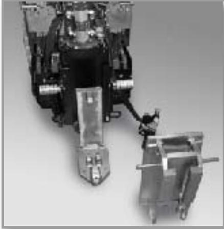
9. Lift the frame out of the machine.
